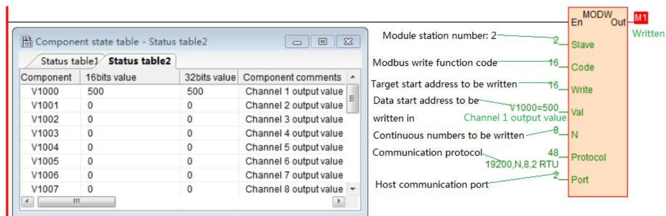
Host PLC writes the 8-channel analog output values of S08AO by Modbus write instruction MODW, the start address is 10H(hexadecimal), that is, the decimal value is 16. When writing successfully, M1 is ON, the 8-channel values which will be written into are stored in V1000-1007.
