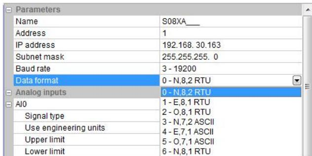
In the external analog input area, we can set the signal type of each channel, choose whether to use engineering value or not, the upper and lower limits of engineering value(it can be set if you check the use of engineering value), sampling times and zero correction.
